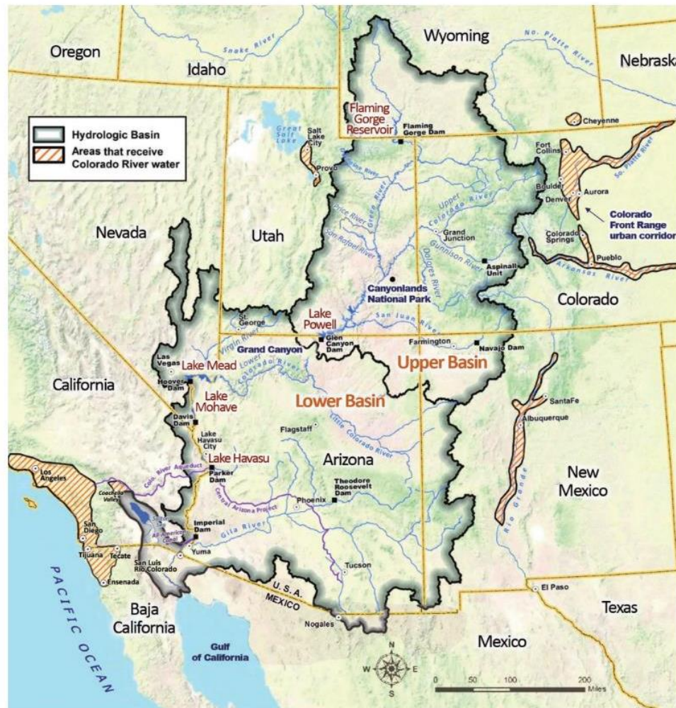
Figure 1. Map showing the watershed, or hydrologic basin, of the Colorado River and areas beyond the watershed that are served by trans-basin diversions (adapted and revised from U.S. Bureau of Reclamation, 2012).
